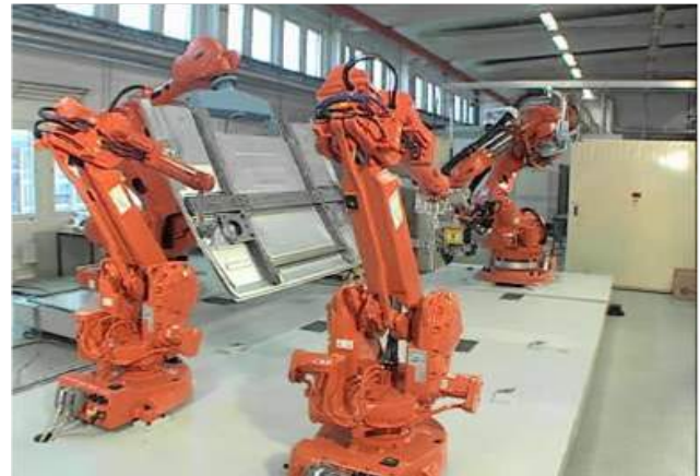
Figure 8: Four collaborating robots controlled according to the ABB MultiMove concept. One robot handles the work object while the 3 other robots simultaneously (and coordinated) perform different processes on the work object.
