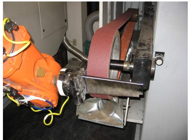
Figure 11: Example of installation using force controlled grinding of a turbine blade.
