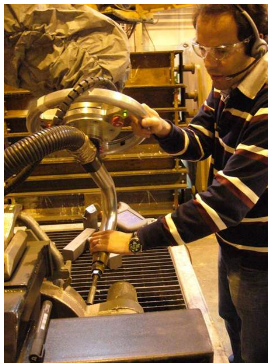
Figure 6: Lead through programming of cutting of a steel casting (using an oxy-fuel burner). The operator makes use of both hands to control the position and orientation of the tool while speech communication is used to define the robot tasks. A 6 DOF force/torque sensor between the tool and the robot wrist is included in a feedback loop to control the tool to move according to the intentions of the operator. The wheel contains distributed safety switches making it possible for the operator to have access to the safety system from all directions.
