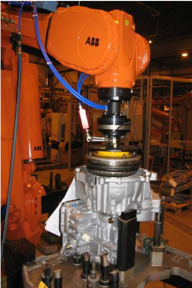
Figure 10: Example of installation using force controlled assembly of a torque converter.
