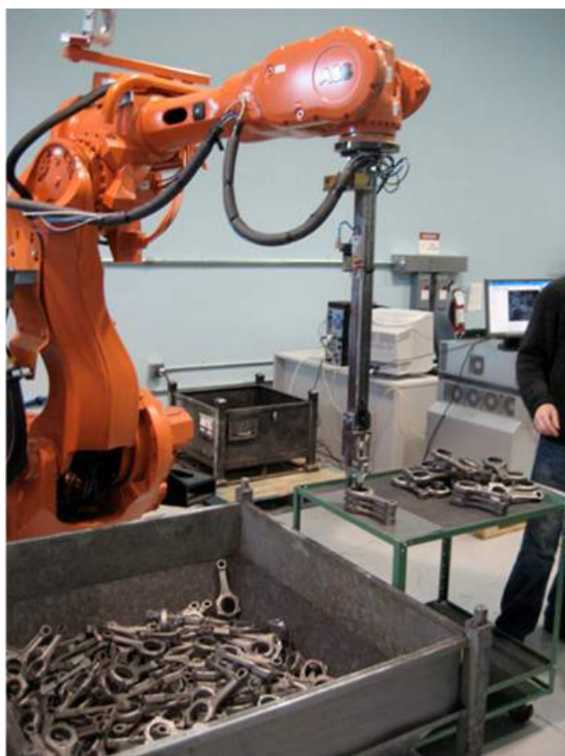
Figure 9: Example of test installation for bin-picking. The gripper is here placed on a long beam to be able to reach the objects everywhere in the deep bin without collisions with the bin walls and without getting too close to singularities.
